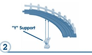
• Fit the "Y" support onto the bottom of the curved ramp track.
